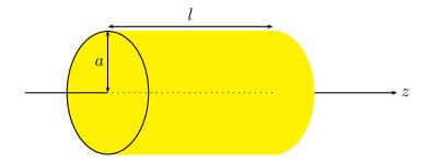
Figure 2: Hollow cylinder (radius a and length l) containing uniform gas flowing along the axis, the z direction, with velocity v. Protons are injected into the cylinder with velocity V parallel to the axis. As a result of magnetic forces, they are brought to a focus at a point on the z axis a distance p far from the cylinder,  $p \gg l$ .
