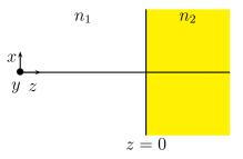
Figure 1: Plane wave normally incident on a surface separating two dielectric materials at z = 0. The medium in the region z < 0 has index of refraction  $n_1$  while the material in the region z > 0 has index of refraction  $n_2$ .
