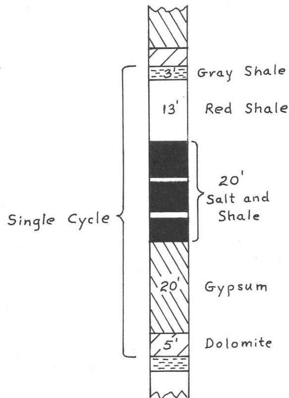
Figure 5. Idealized complete cycle of evaporite deposition in the Flowerpot, Blaine, and Dog Creek Formations of north-central Texas.
