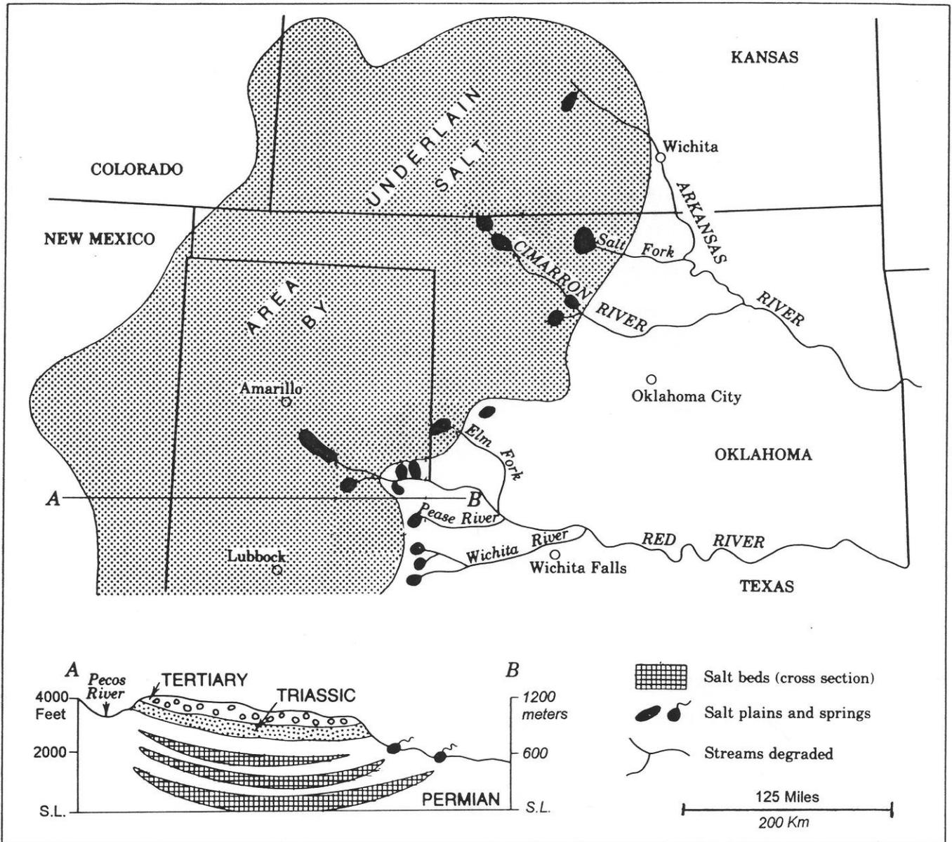
Figure 1. Map and schematic cross section showing distribution of Permian salts and salt plains in the Red River and Arkansas River watersheds of western Oklahoma and adjacent areas (Johnson, 1981).
