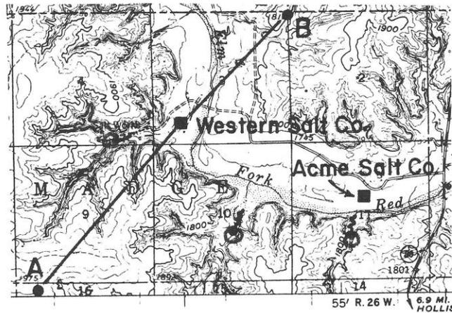
Figure 9. Generalized cross section (above) and location map (below) showing salt layers, brine springs, and stratigraphy in the vicinity of Salton (or Chaney) Salt Plain on Elm Fork Red River (from Johnson and Denison, 1973). In 1973, two companies (Western Salt Co. and Acme Salt Co.) were producing solar salt from evaporating pans on the Elm Fork alluvial plain.
